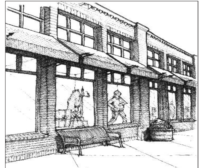
Figure 27 -- Ground floor display windows and "divided lights" above.
