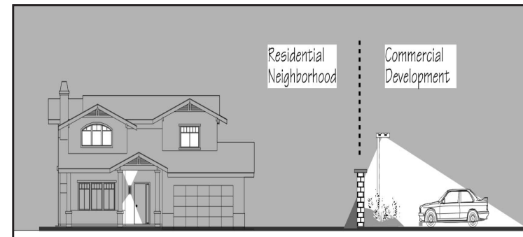
Figure 77 -- Commercial development should be designed to protect privacy and minimize nuisance impacts to adjoining residences
