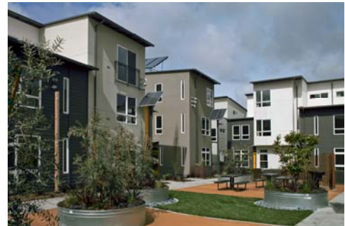
Internal courtyard for residents shielded from traffic noise by the building mass surrounding it.
