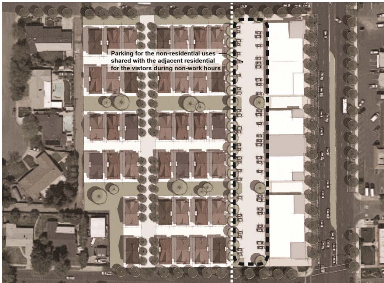
Figure 5-6: Site layout showing shared-parking between residential and non-residential uses on adjacent sites.
