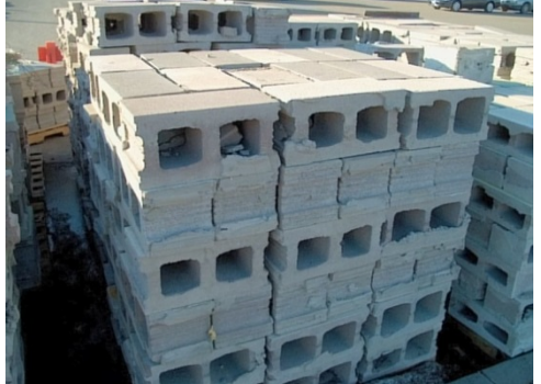
Use appropriate material specifications, such as concrete blocks, double or triple-pane windows help to reduce noise level from Highway into the interiors of the buildings
